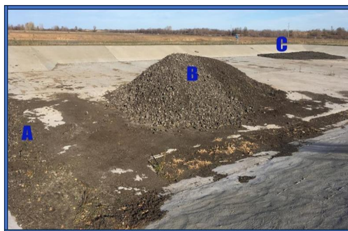
Fig. 1 The sludge sediments were found in a pit located within the West Kazakhstan region. Sampling sites for silt sediment at various stages of natural dehydration in different years: Sediment from 2015-2016 was collected at point A; Sediment from 2017-2018 was collected at point B; Sediment from 2019 was collected at point C.
