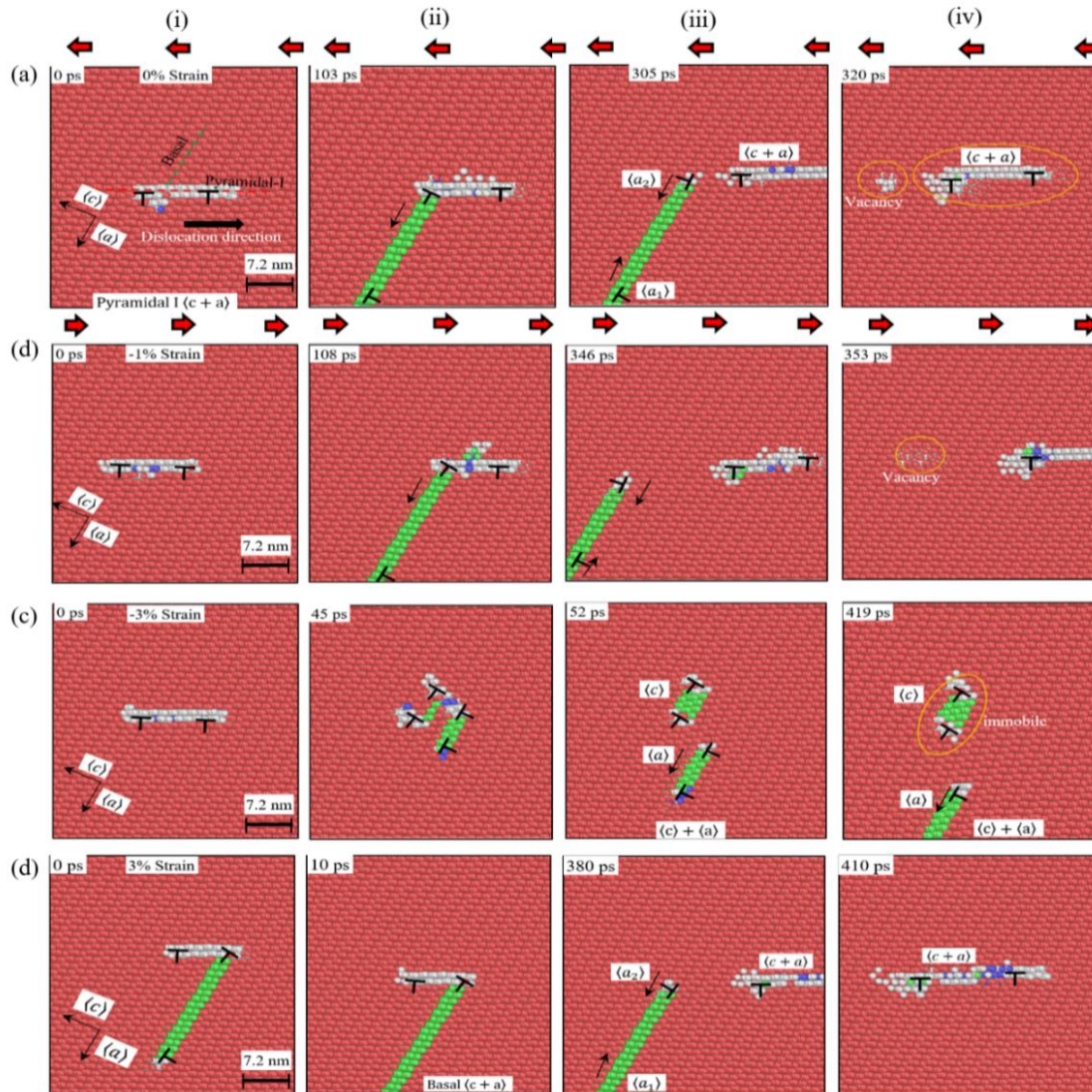
Fig. 4 Glide behavior of a Pyr-I \langle c + a \rangle edge dislocation at 10 K, as observed during long-time MD simulations, under shear deformation for normal strains of (a) 0%, (b) -1\% , (c) -3\% , and (d) 3\% . The direction of the shear deformation is shown by the arrows in (a) (a color version of the image is available online).
