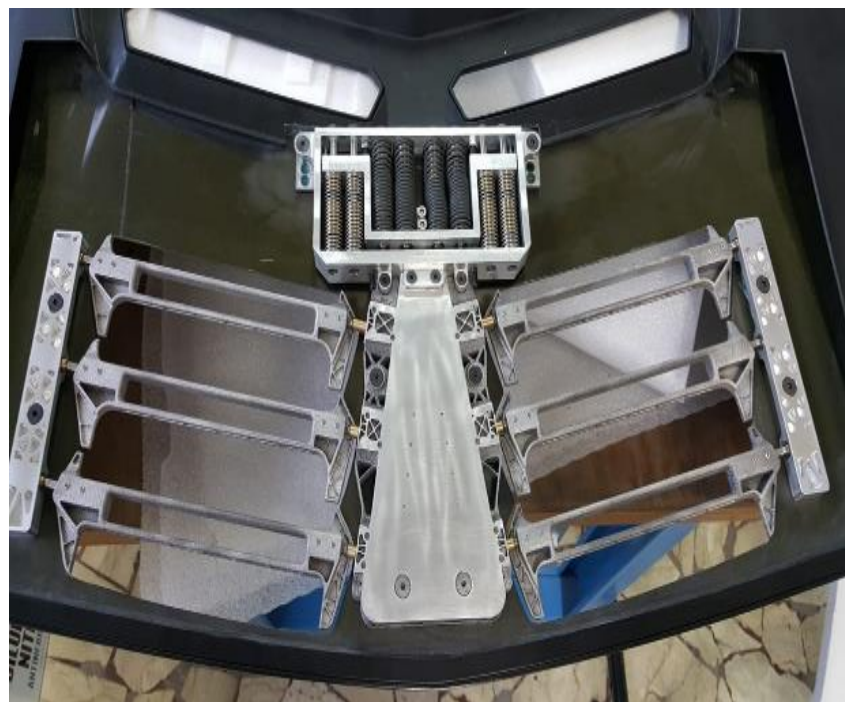
Fig. 30 SMA-based cooling system device installed on the rear bonnet.
