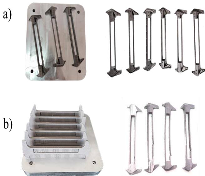
Fig. 23 Flap supports a) improperly and b) correctly printed.
