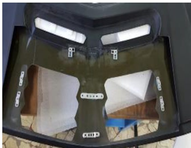
Fig. 29 Supports glued on the rear bonnet.
