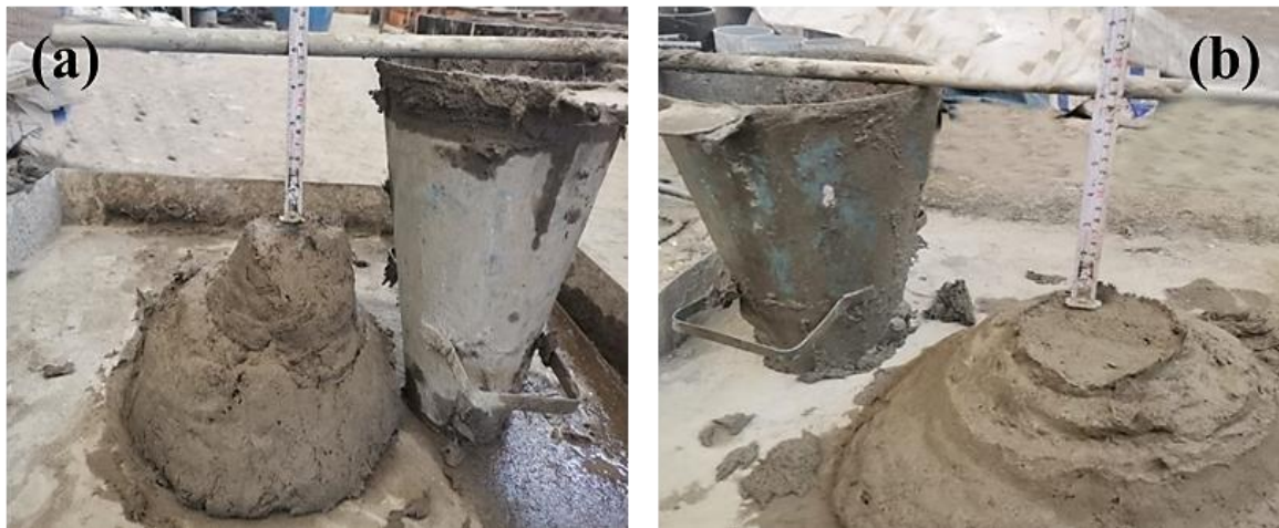
Fig. 8 Slump test types; (a) Shear slump, and (b) Collapse slump.
