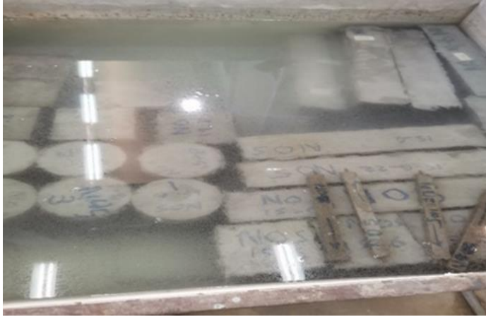
Fig. 4 Concrete specimens in curing water tank.
