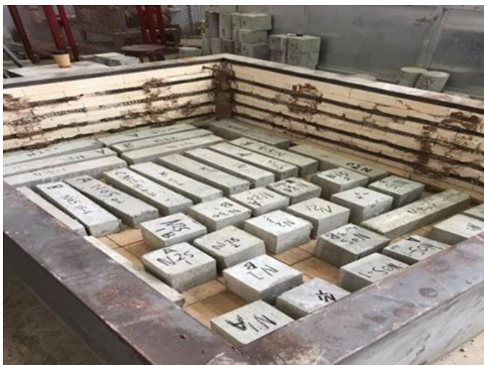
Fig. 6 Arrangement of specimens inside the furnace.
