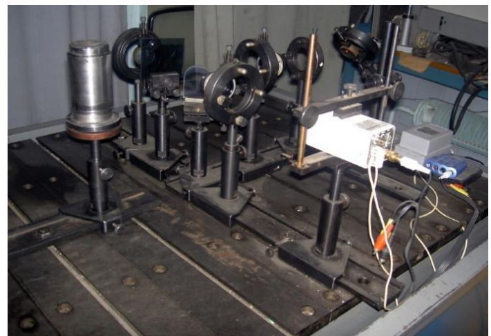
Fig. 3 Experimental installation for detecting residual stresses in the metal coating layer using the penetration method.
