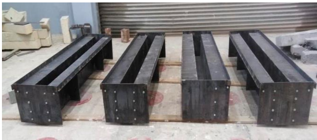
Fig. 2 Steel formwork used in casting the T beams.
