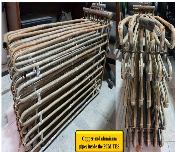
Fig. 4 The experimental setup of the PCM TES.
