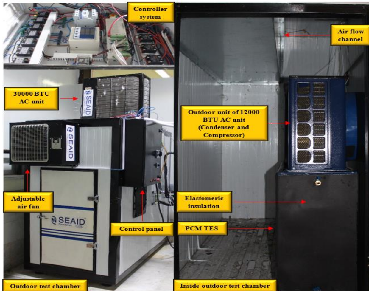
Fig. 1 The experimental setup of the outdoor test chamber with its equipment.
