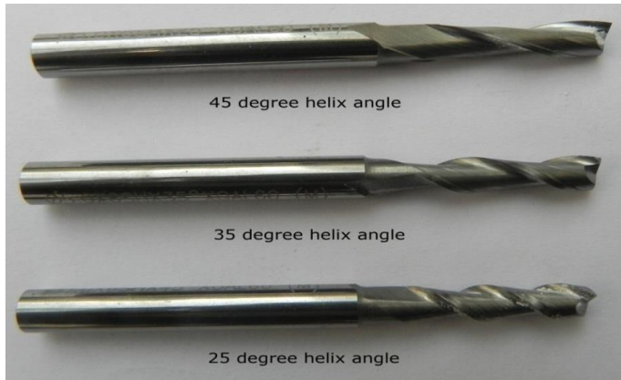
Fig. 2 Solid carbide end mill with different helix angles.
