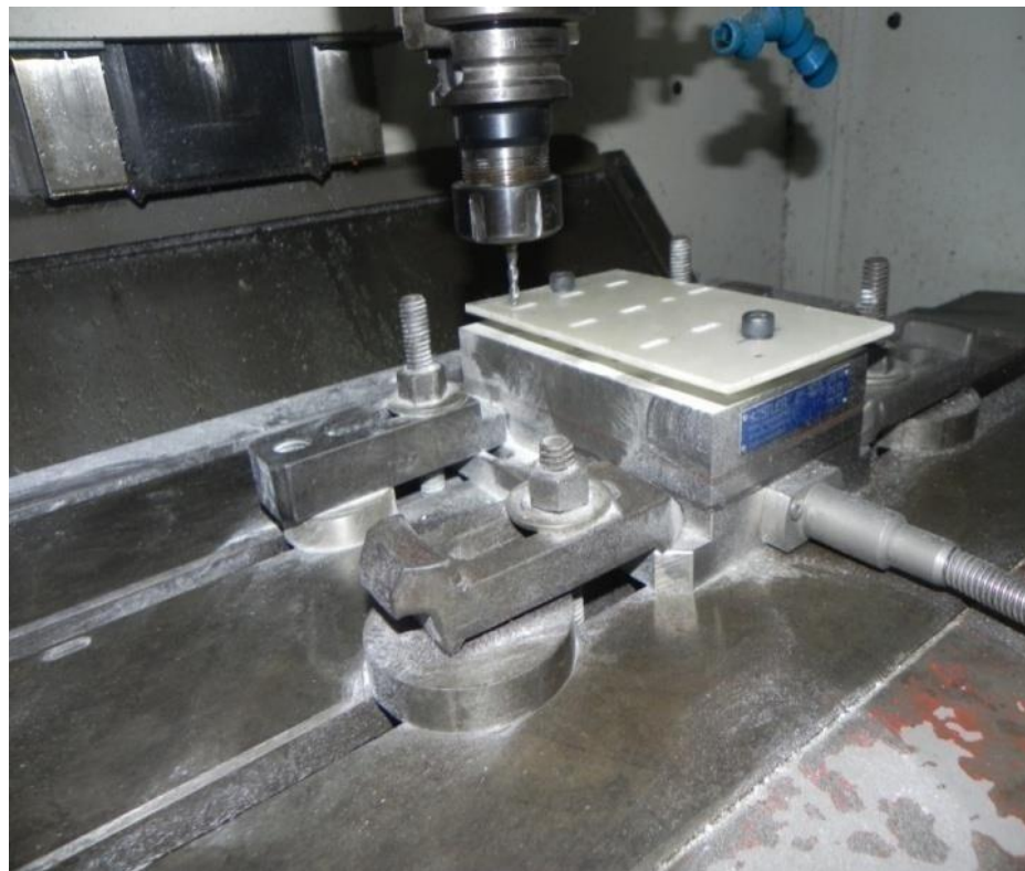
Fig. 3 Fixation of GFRP composite plate by using clamps in the machining centre.
