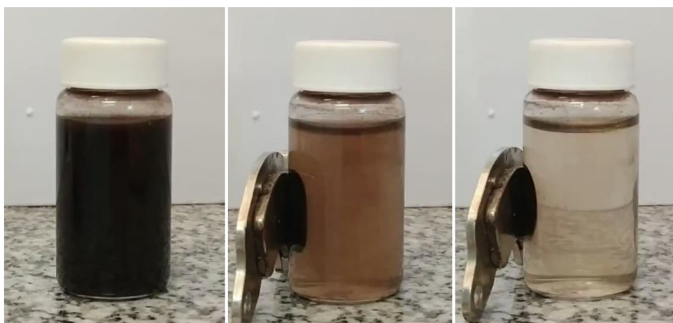
Fig. 4 Magnetic separation of NP-Ch with commercial permanent magnet (NdFeB).
