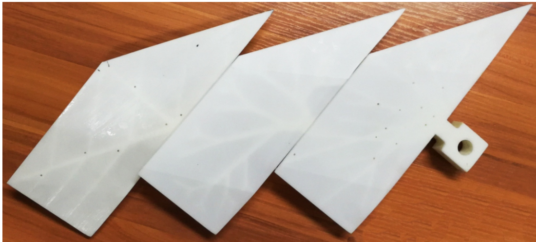
Fig. 14 Three different designs fabricated with stereolithography based resin additive manufacturing.
