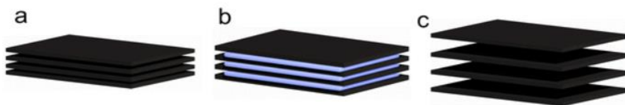
Fig. 7 Activation mechanism by the penetration of metallic K into the a) carbon lattices, the expansion of the lattices by the b) intercalated metallic K, and the removal of the intercalated K from the c) carbon matrix. Reproduced with the permission from [69], Copyright Royal Society of Chemistry.
