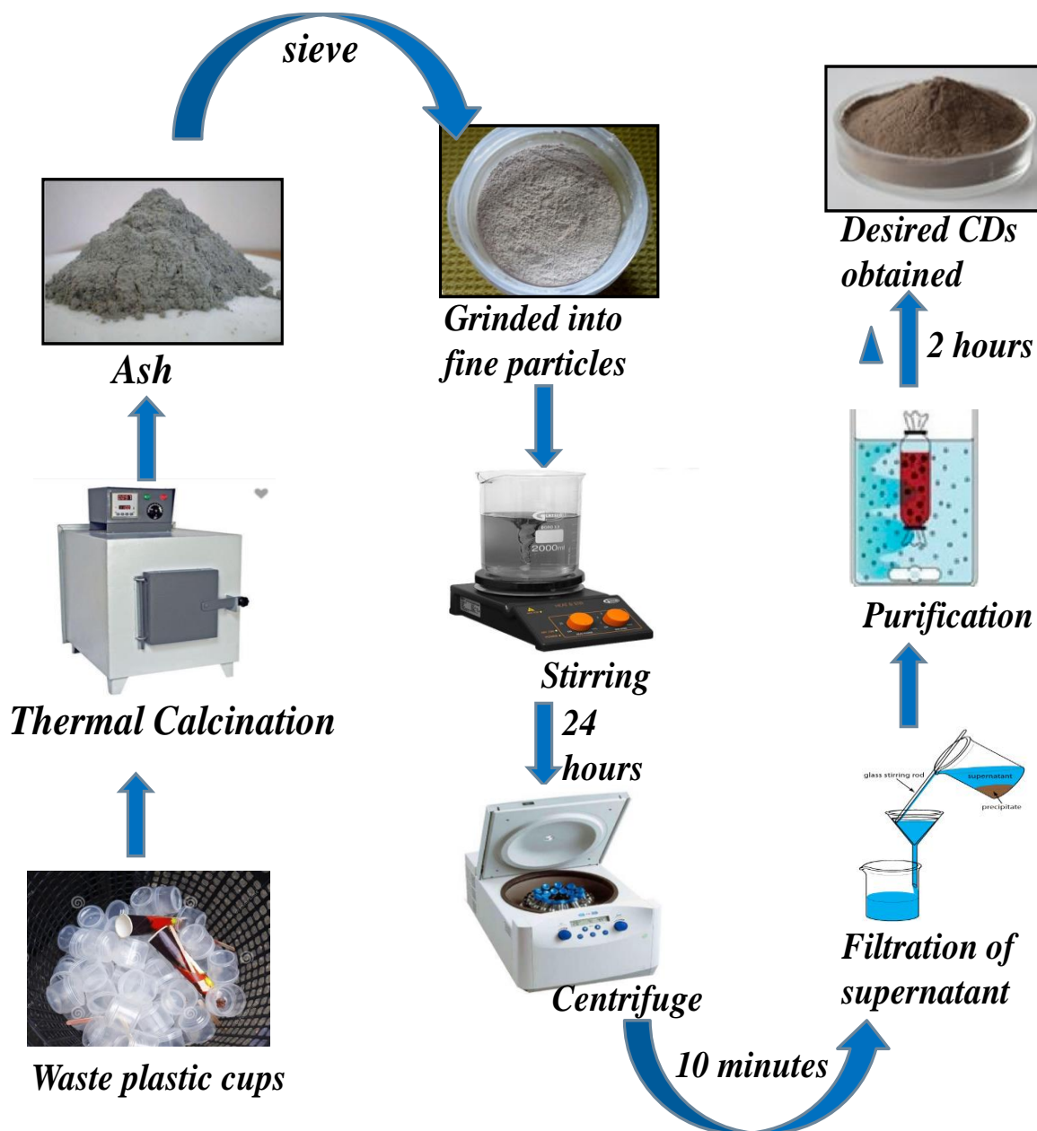
Scheme 1. Schematic illustrations showing the synthetic route of CDs from waste plastic cups.
