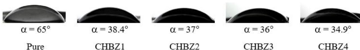
Fig. 6 Images of drop on biopolymer nanocomposite under different weight fractions of ZrO 2 .
