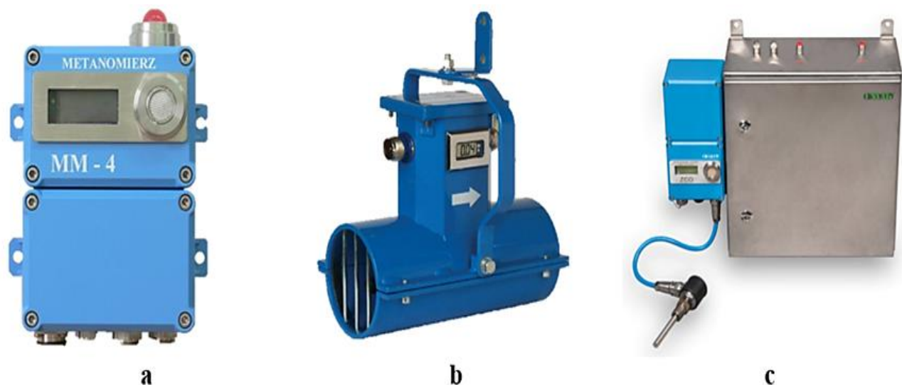
Fig. 5 Sensors of the methane gas system in the studied region (a - methanometer, b - anemometer, c - integrated drainage sensor).
