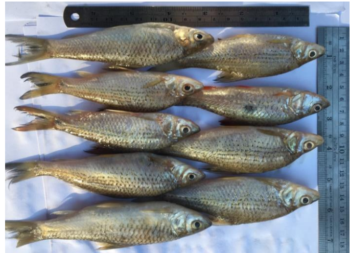
Fig. 6 The characteristics of the scaled fish obtained by the proposed machine.
