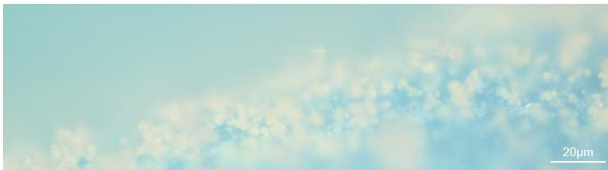
Fig. 6: Steel edge corrosive pitting after 5% Na 2 SO 4 immersion for 24 h.
