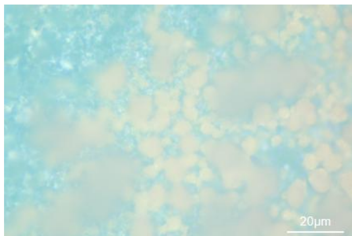
Fig. 3: Structural diagram of the steel corrosion products after artificial seawater immersion for 24 h.
