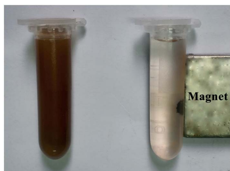
Fig. 5 The photographs of Corrole-Fe 3 O 4 suspension in water before and after exposure to a magnet.
