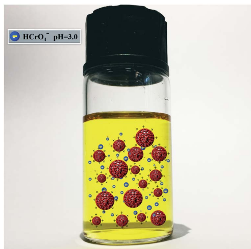
Fig. 6 Proposed adsorption mechanism of Cr(VI) by FC515 in optimal adsorption condition.
