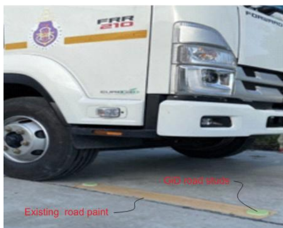
Fig. 9: Field trial with a vehicle cyclic tire loading test. (Real world field test setup, and schematic diagram of test mechanism).
