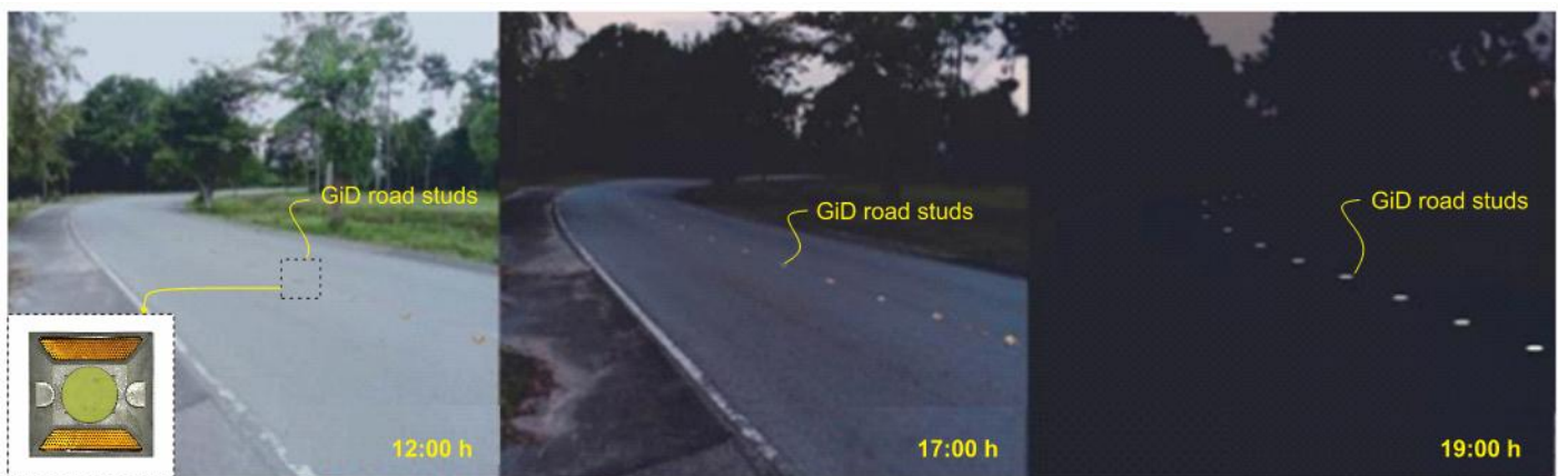
Fig. 15: Photos of GiD studs on rural road of walailak university at 12:00 h, 17:00 h and 19:00 h.
