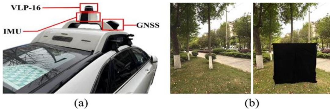
Fig. 8: The experiment setup. (a) AV platform (b) Light-absorbing material deployment: Original scene (left), Region hidden scene (right).
