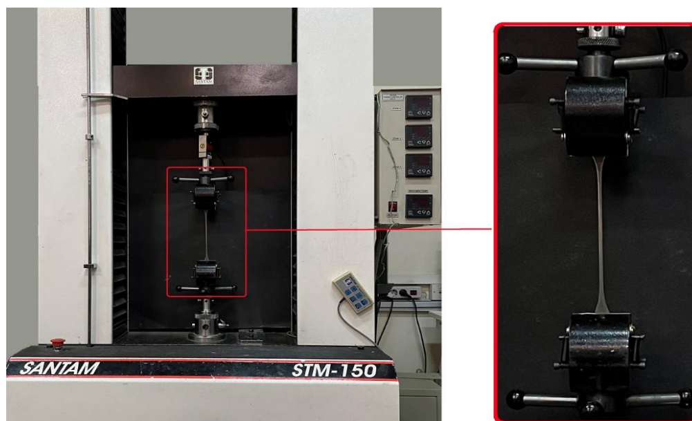
Fig. 5: The tensile testing of a specimen.
