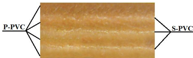
Fig. 7: The cross-section view of Laminate-2.
