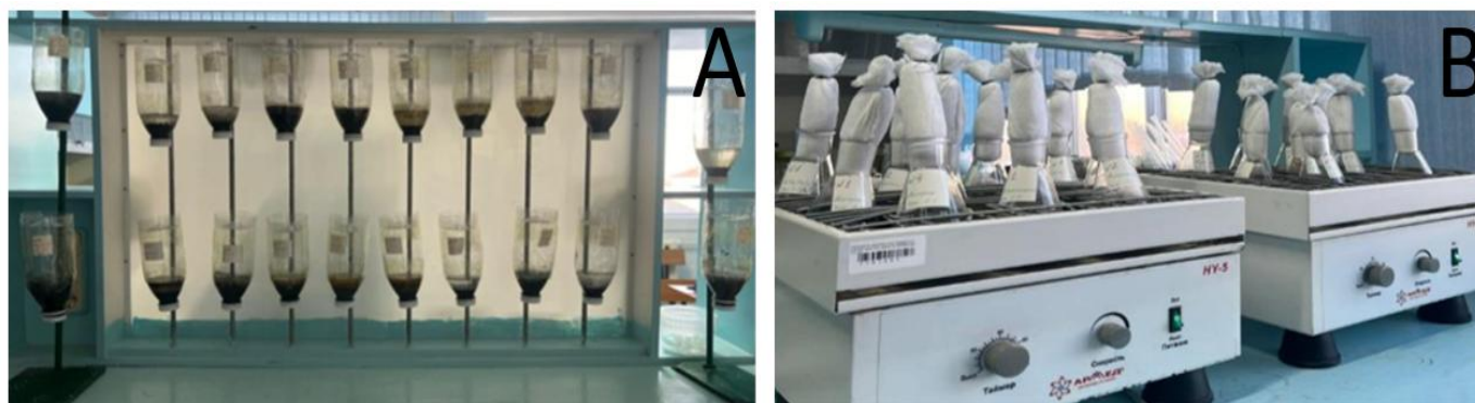
Fig. 2: Setups for bioleaching in laboratory conditions: A. Laboratory setup simulating heap leaching ; B. Laboratory setup simulating tank leaching.
