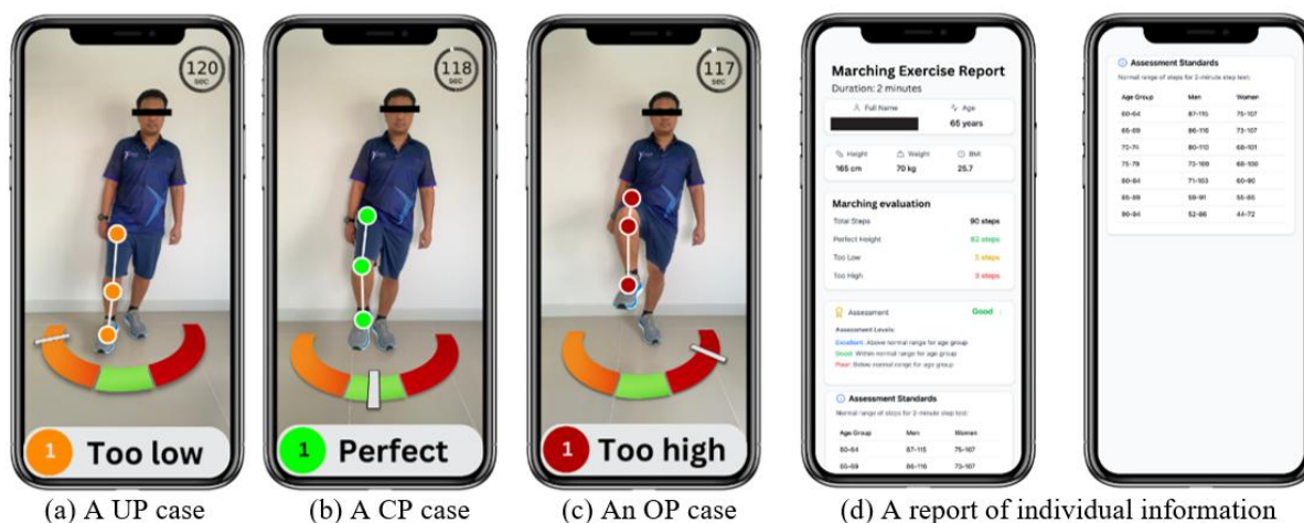
Fig. 5: An application AR posture guidance system for the elderly two-minute step test based on marching exercise based on the correct, over, and under posing evaluated by \theta .
