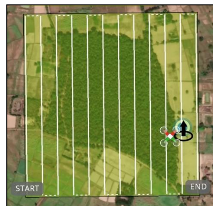
Fig. 3: UAV flight path design and aerial data acquisition for detailed image-based mapping of the survey area.
