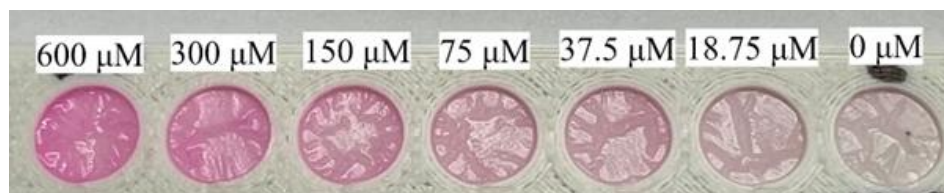
Fig. 7: Visual quality of the readout from hydrogel-based uric acid assay.
