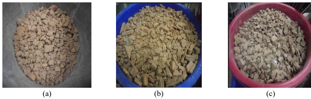
Fig. 5: Recycled brick aggregates originated from brick: (a) CBA, (b) CBB, and (c) CBC.
