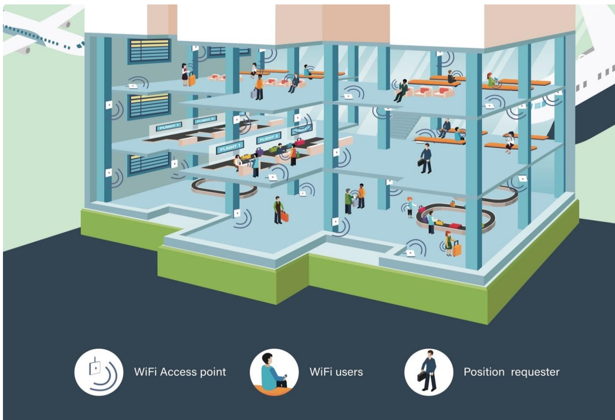
Fig. 1 The schematic application of WiFi based indoor localization in an airport.
