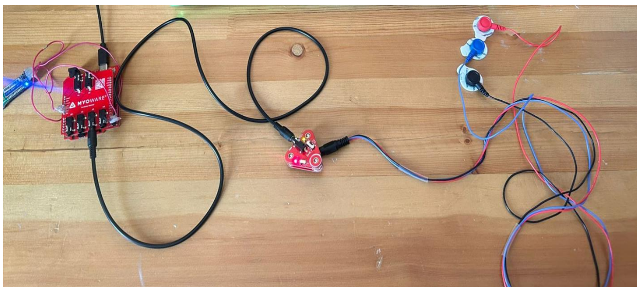
Fig. 3 MyoWare 2.0 sensor for electromyography signal detection.
