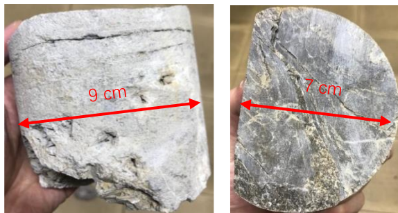
Fig. 2 Photos of the dolomite core from depth 4285.7 – 4286 m.
