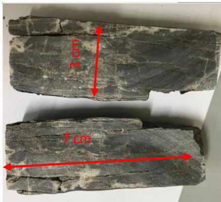
Fig. 3 Cut dolomite core sample from depth interval 4,285.7 – 4286 m.
