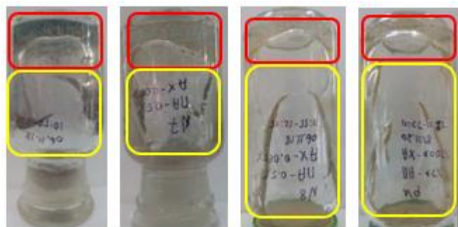
Fig. 10 0.5 % 6-7 mln Da 5 % HD HPAM / 0.1-0.0125 % (decreasing from left to right) chromium acetate in sea brine. Chromium acetate concentration decreases from left to right. Red rectangle – strong gel. Yellow rectangle – tonguing gel.
