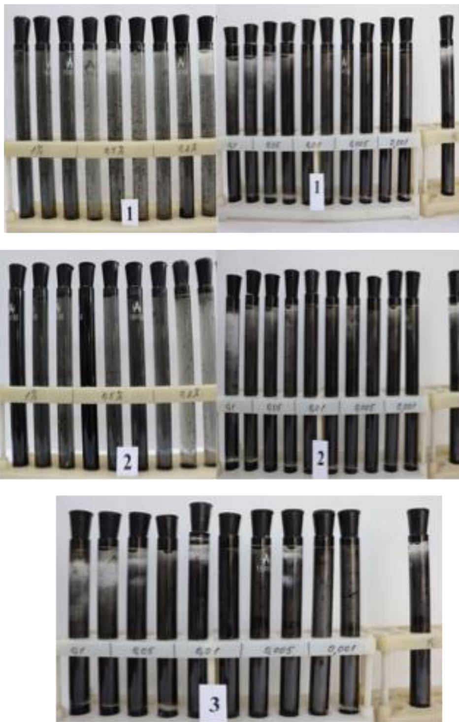
Fig. 10 Growth of sulfate-reducing bacteria (SRB) in the presence of various concentrations of [TMAPMACH]:[DMAA] copolymers with different monomer ratios: (1) [TMAPMACH]:[DMAA] (mol.%) = 40:60; (2) [TMAPMACH]:[DMAA] (mol.%) = 50:50; (3) [TMAPMACH]:[DMAA] (mol.%) = 60:40. The rightmost sample, labeled as K, represents the control variant where SRB was cultured without the copolymer.
