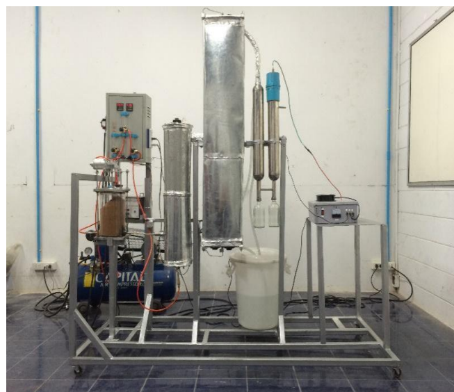
Fig. 2 Fast biomass pyrolysis using a fluidized-bed reactor unit.
