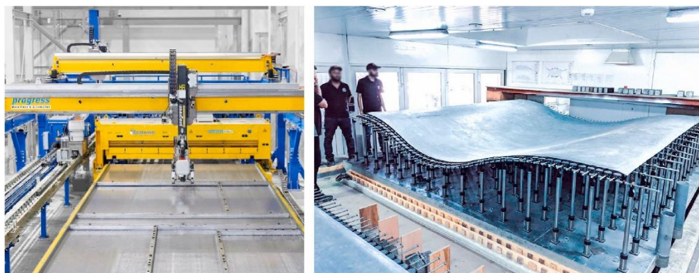
Fig. 18 Robotic formwork system with a shuttering robot. Reproduced with the permission from [158], Copyright 2021 The Author(s).
