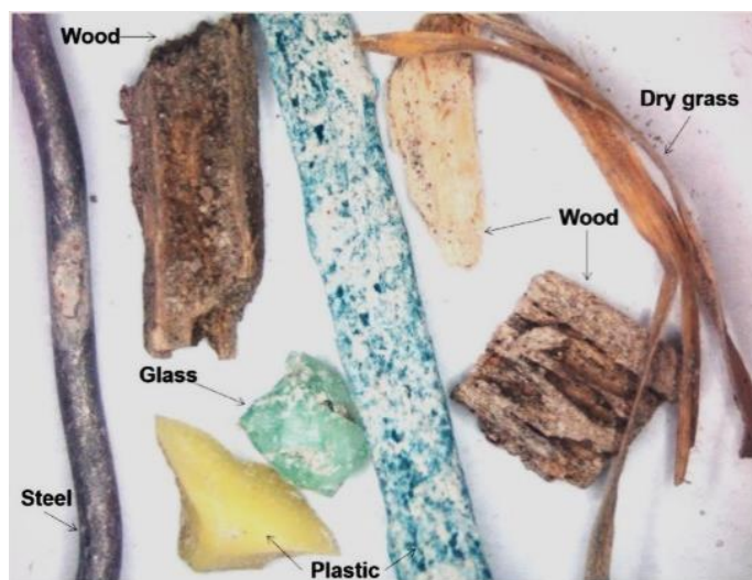
Fig. 8 Contaminants in FRCA. Reproduced with the permission from [95], Copyright 2021 The Author(s).
