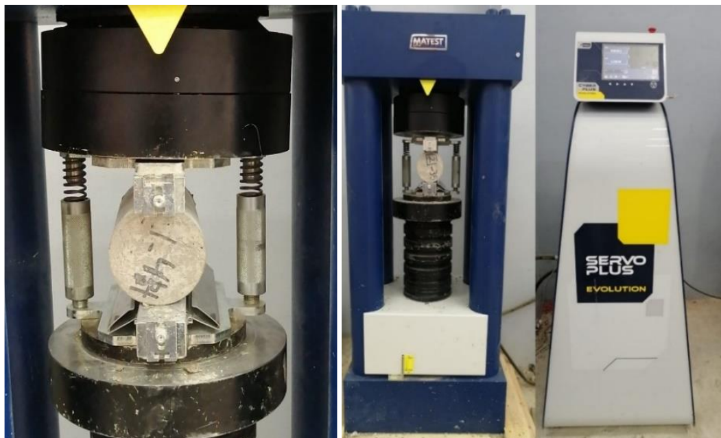
Fig. 8 Splitting Tensile strength test machine.
