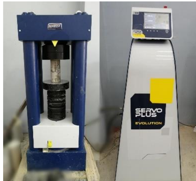
Fig. 7 Compressive strength test machine.
