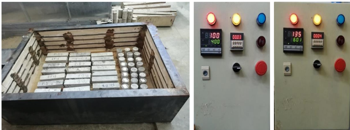
Fig. 13 The samples before being subject to the high temperatures in a furnace and the external display shows the target temperature (400 °C and 600 °C).
