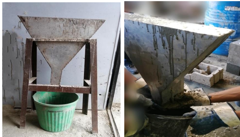
Fig. 5 Steps of the V-funnel test.
