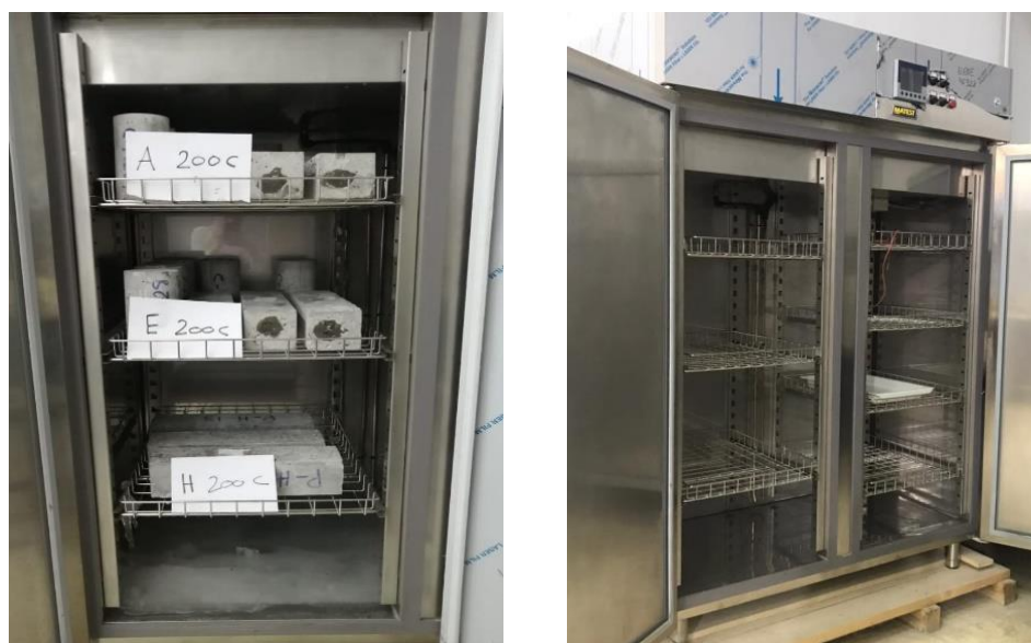
Fig. 12 Freeze-Thaw chamber and Specimens before being subjected to freeze-thaw cycles.
