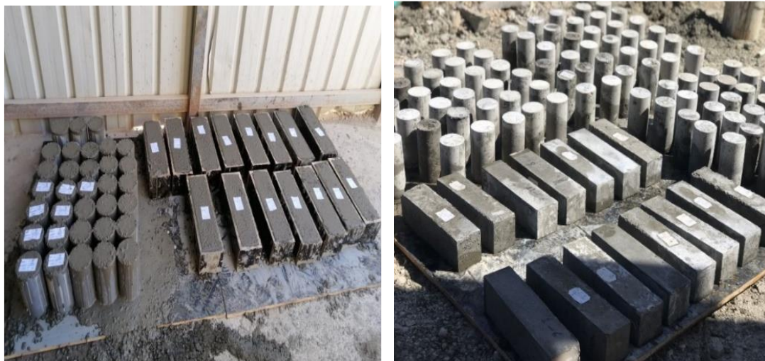
Fig. 2 Procedures for casting and curing specimens.
