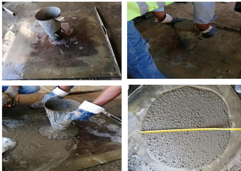
Fig. 3 Steps of the slump flow test.
