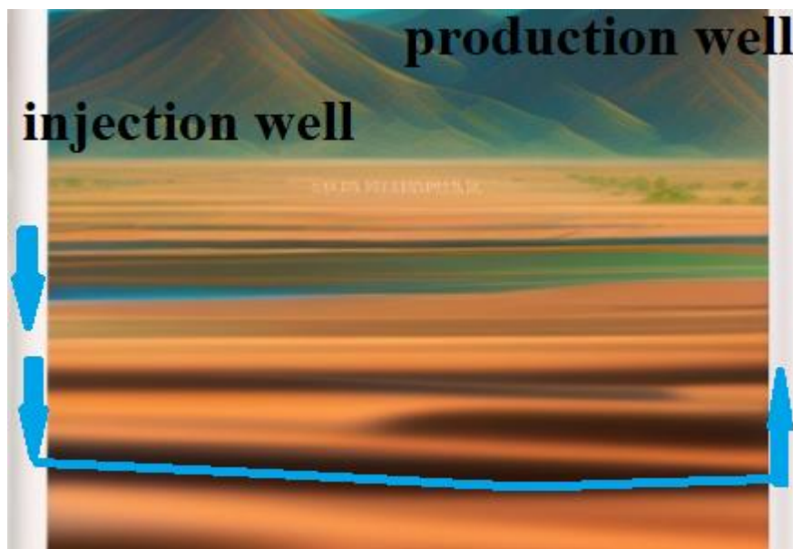
Fig. 1 Movement of water from a reservoir pressure maintenance system in an oil reservoir.
