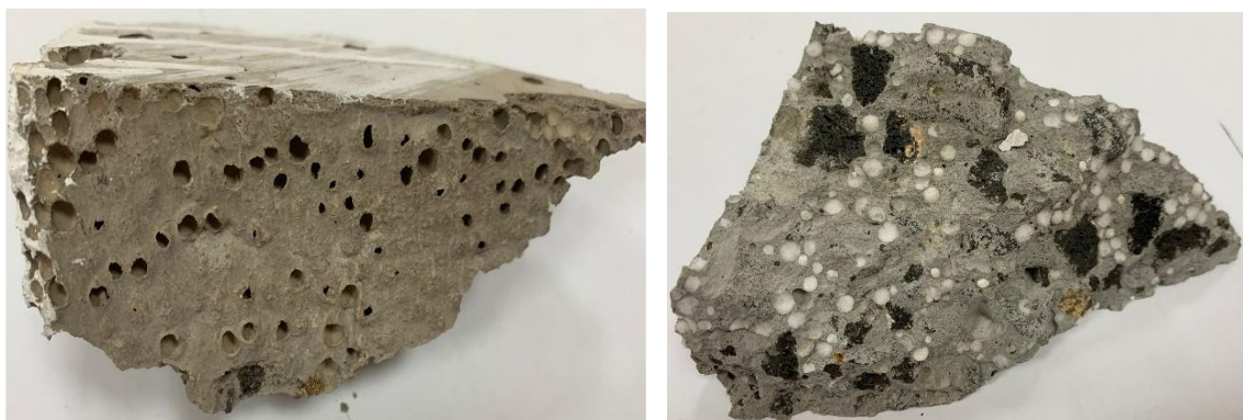
Fig. 13 The influence of temperature on EPS beads on the surface and inside the RC beams.
