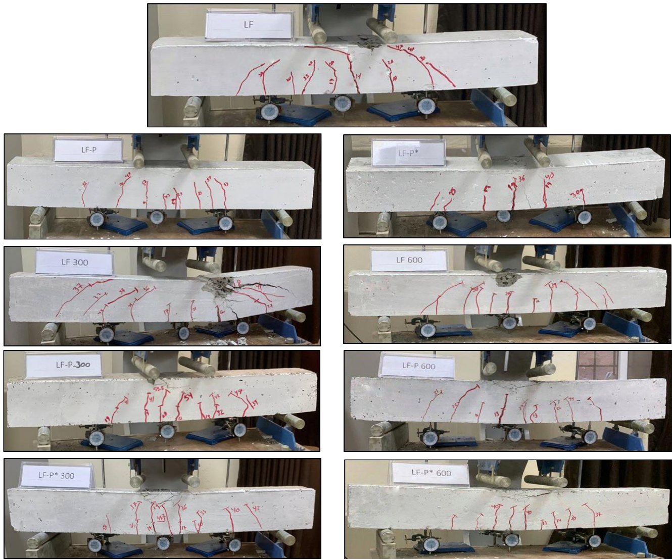
Fig. 12 Crack patterns of tested beams.
