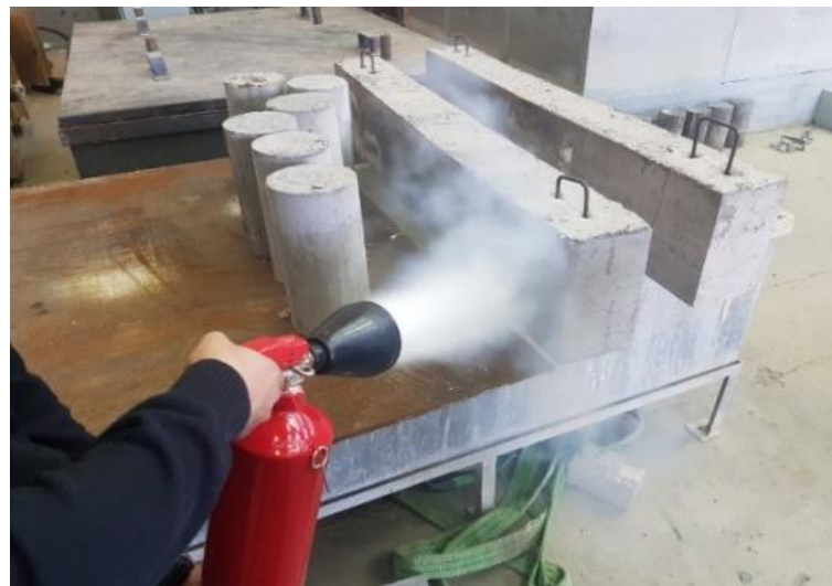
Fig. 9 Placement of specimens into water and Cooling of specimens using a CO 2 fire extinguisher.
