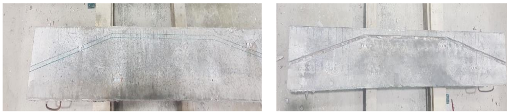
Fig. 10 Outlining the grooving perimeters and Grooving using a rotary saw blade.
