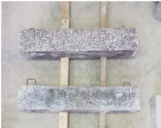
Fig. 16 Spider web cracks caused by heat-shock.
