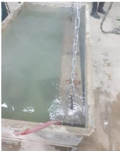
Fig. 9 Placement of specimens into water and Cooling of specimens using a CO 2 fire extinguisher.
