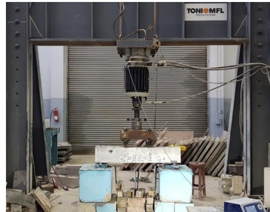
Fig. 13 Flexural test setup.
