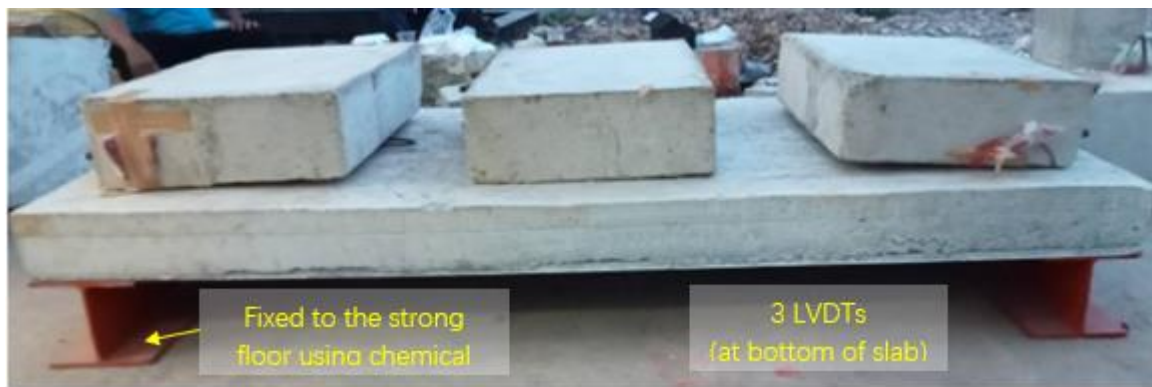
Fig. 5 Typical experimental setup for sustainable loading tests.
