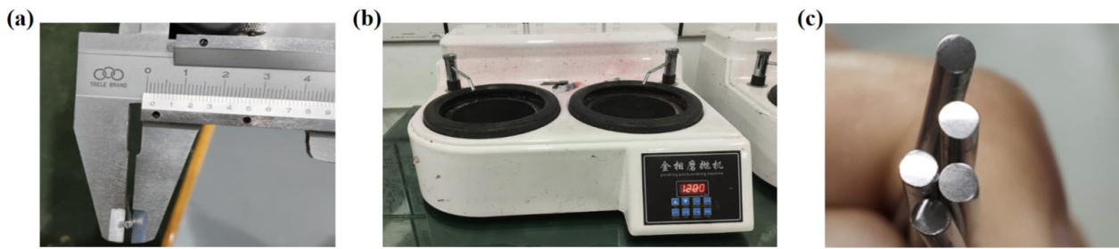
Fig. S1: (a) Hot-dip galvanized steel wire diameter as measured, (b) Metallographic grinding and polishing machine, (c) Steel sample preparation.
