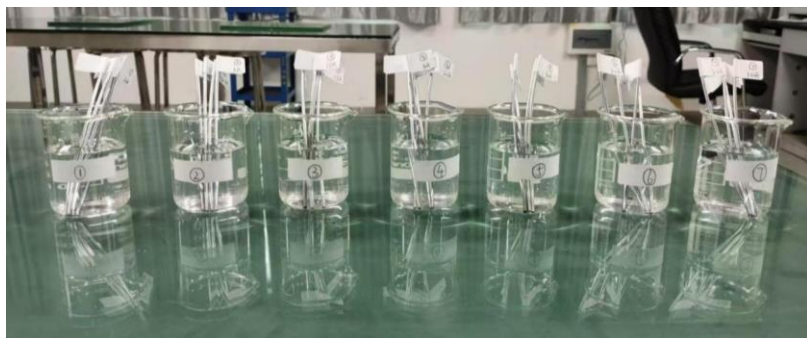
Fig. S2: Initial solutions in the immersion corrosion test.
