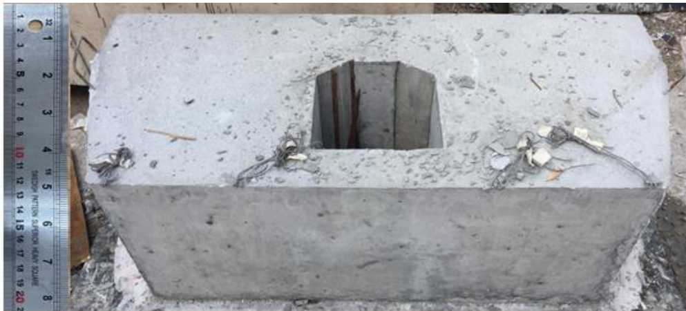
Fig. S2: Typical pier segment after curing period.
