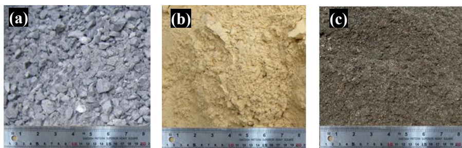
Fig. S1: Fine aggregate in this study: (a) crushed rock fines, (b) diatomite, and (c) sugarcane bagasse ash.
